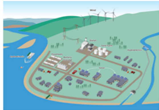
Figure 1. Illustration of a Microgrid
