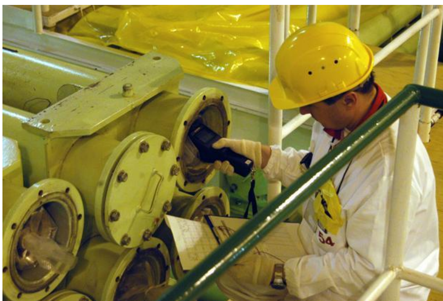
IAEA Safeguard inspector scanning fuel assemblies in Mochovce nuclear power plant in Slovakia.
